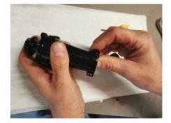
If you have the experience: remove the seal, clean the bearing and apply SKF bearing grease. If needed change the bearing.
