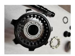
Place the bearing seal back in position.
