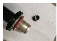
Remove the floating ring and inspect the springs and their condition, clean them and apply new grease.
