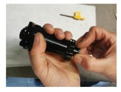
Use a spanner if needed, but do not use excessive force to open both ends.
